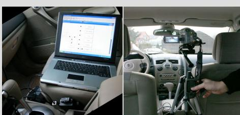
Complex of measuring devices in the instrumented car, in the left picture there is possible to see the view as it was recorded on the camera.
